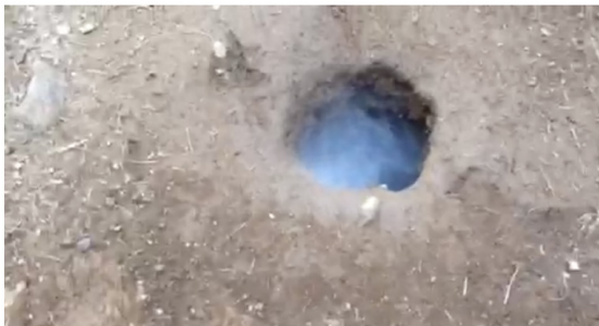
Figure 4. Propylene glycol fog emerging from a connected burrow. Propylene glycol vapor was pumped into a single burrow entrance and then all other burrows were monitored for emerging fog. Burrows found with emerging fog were documented as having a direct physical connection with the origin burrow.
